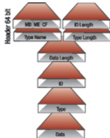
FIGURE 3 ID, Type, and Data starts on 32-bit boundary
